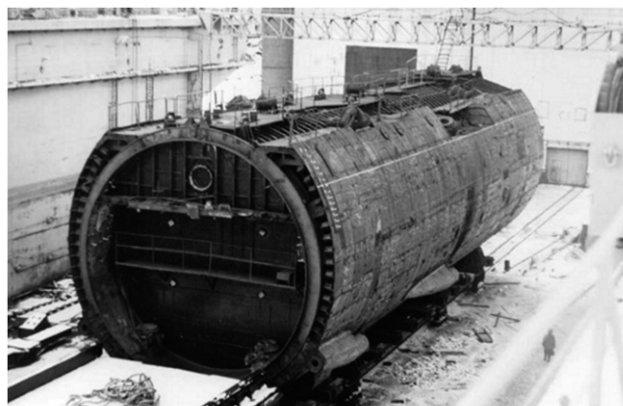
Fig. 1. Reactor compartment of a cruiser submarine.
